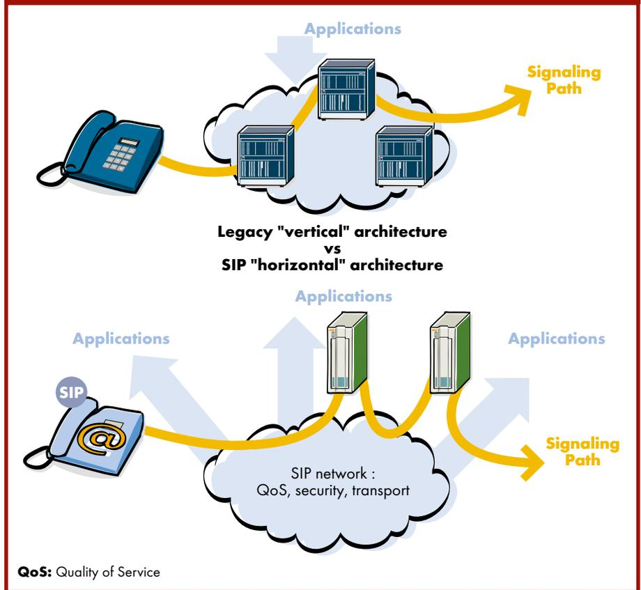
SIP goes beyond the scope of VoIP to provide building blocks for new enterprise communication applications:
